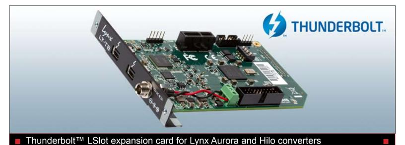
The LT-TB is an LSlot expansion card for the Aurora 8, Aurora 16, Aurora 16-VT and Hilo converters that allows daisy-chaining of up to six devices using the Thunderbolt port on Mac and PC Computers
