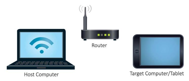
The Host computer must be running LynxRedirector and be <u>directly connected</u> to the Hilo either via USB or Thunderbolt. Additionally, the Host Computer must be connected to your network router either via Ethernet cabling or over Wi-Fi (direct Ethernet cabling will provide the best performance). The Target Computer/Tablet running Hilo Remote must connect to your network router either via Ethernet cabling or over Wi-Fi.
