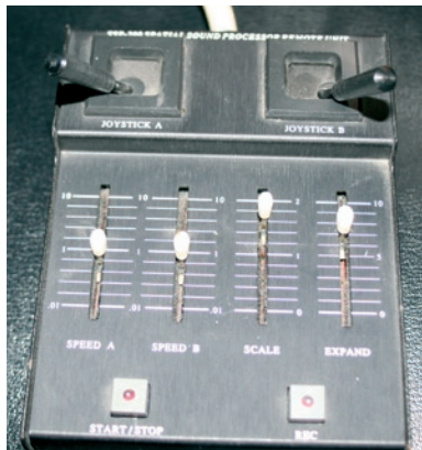
One of the many unusual pieces of gear at Paper VU is the Sensortech SSP200 Spatial Surround Processor, with its joystick-based remote control (right). Beneath it in the rack is the A Designs Hammer EQ which was used extensively on 'Boom Boom Pow'.
