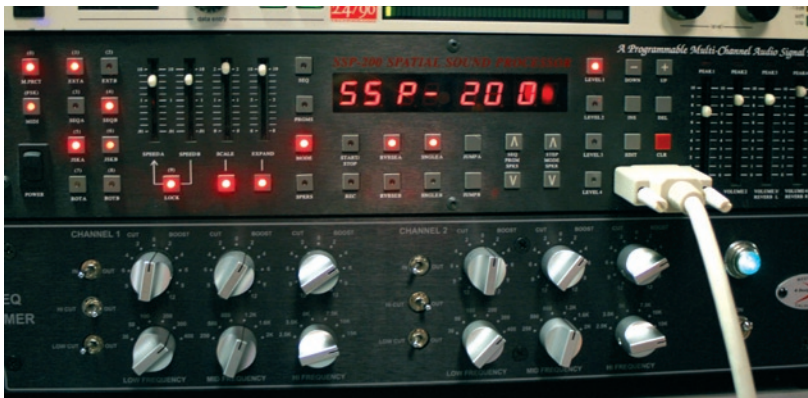
One of the many unusual pieces of gear at Paper VU is the Sensortech SSP200 Spatial Surround Processor, with its joystick-based remote control (right). Beneath it in the rack is the A Designs Hammer EQ which was used extensively on 'Boom Boom Pow'.
